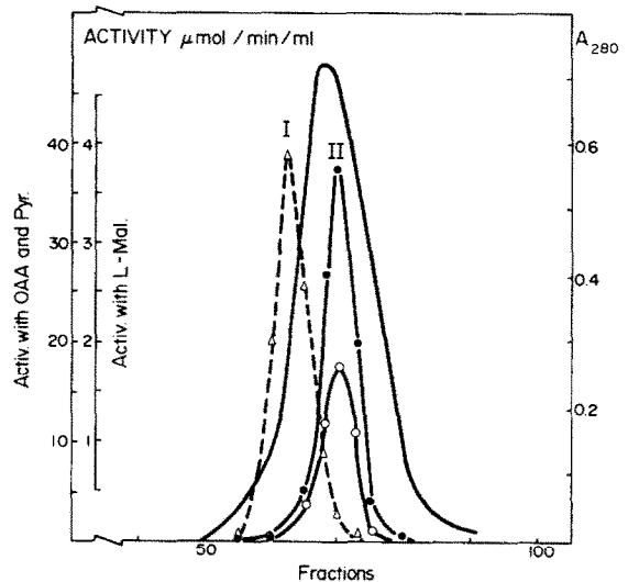
Fig. 6. Elution pattern of cytoplasmic malate dehydrogenase and lactate dehydrogenase obtained in step 3 of the purification procedure (described in Materials and Methods) from Ultrogel AcA 34. The column (2.6 × 100 cm) was equilibrated and eluted with Tris–HCl buffer 0.1 M, pH 8.5 at 4°C. Flow: 35 ml/hr. Activities: (●) with OAA and NADH; (Δ) with pyruvate and NADH; (○) with L-malate and NAD<sup>+</sup>; (—) Absorbance at 280 nm. The fractions collected were 5 ml.
